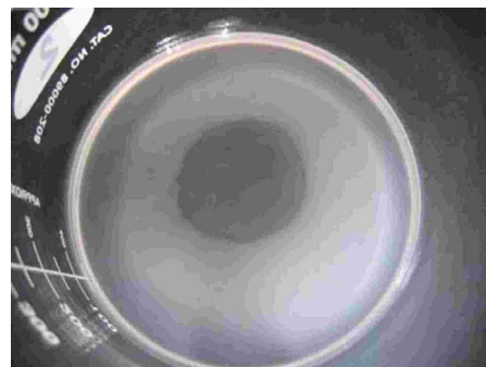
FIG. 2. (Color online) Appearance of a clear cylinder near the center of a glass beaker containing an aqueous suspension of microspheres. Photo taken from top of beaker.
